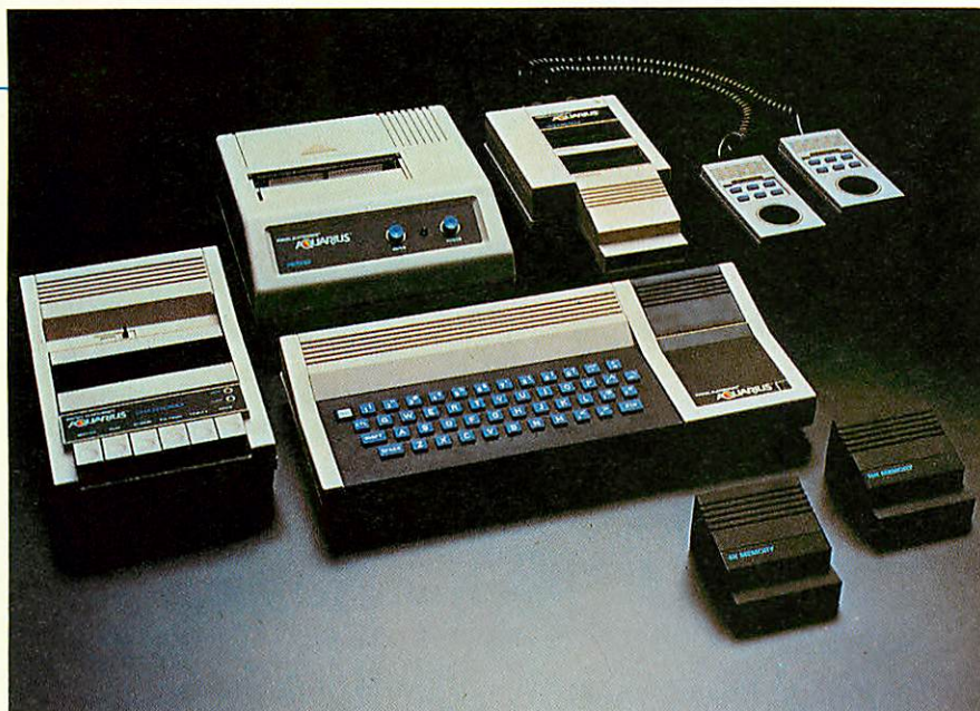
Aquarius computer, with its data recorder, printer, Mini Expander, game controllers, and RAM expansion cartridges
