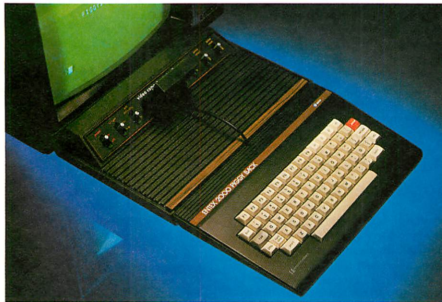
Keyboard adapters that expand the Atari 2600 video game into a home computer are available from Atari (above), as well as from third-party companies (below).
