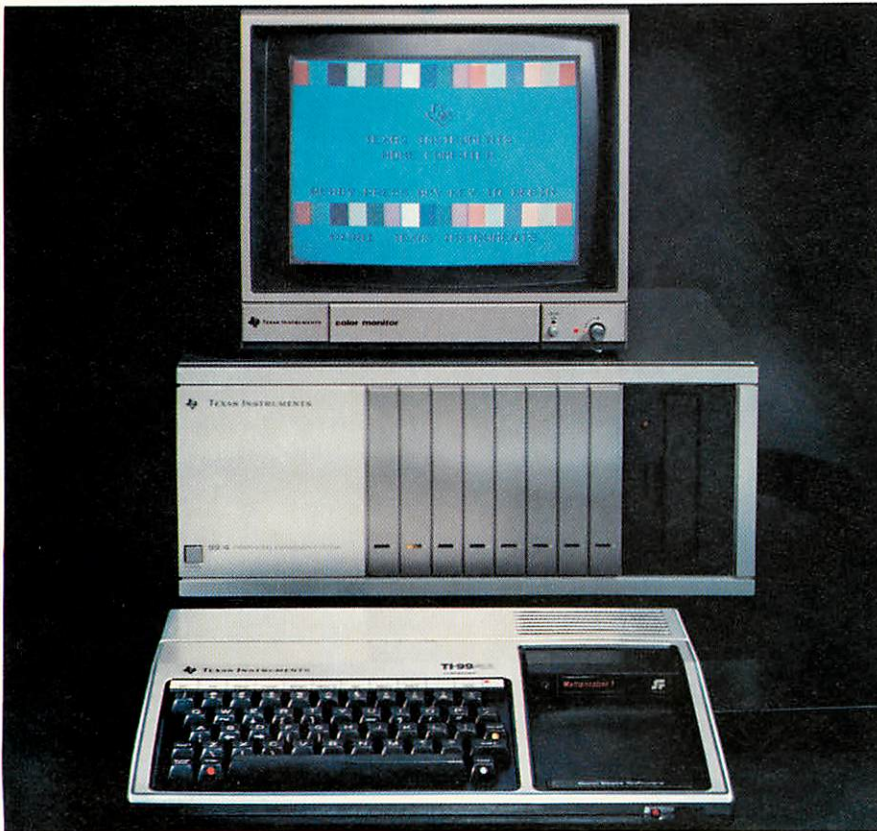
Texas Instruments TI-99/4A computer, with its peripheral expansion system and color monitor
