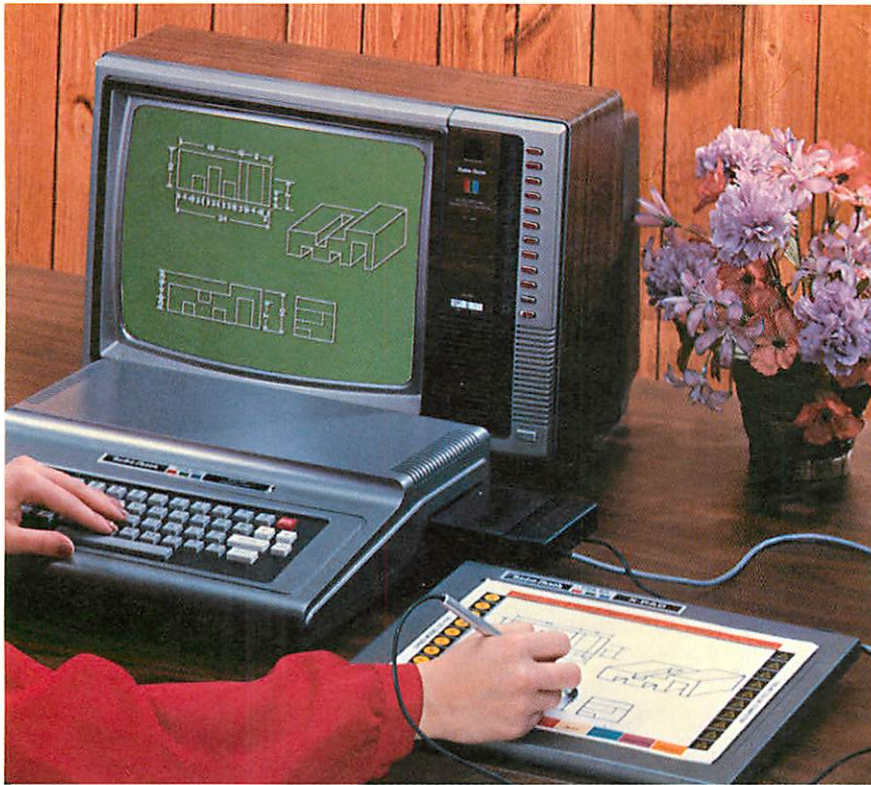
A digitizer can turn you into a computer artist. Lines and shapes drawn on its surface appear like magic on the computer screen.
