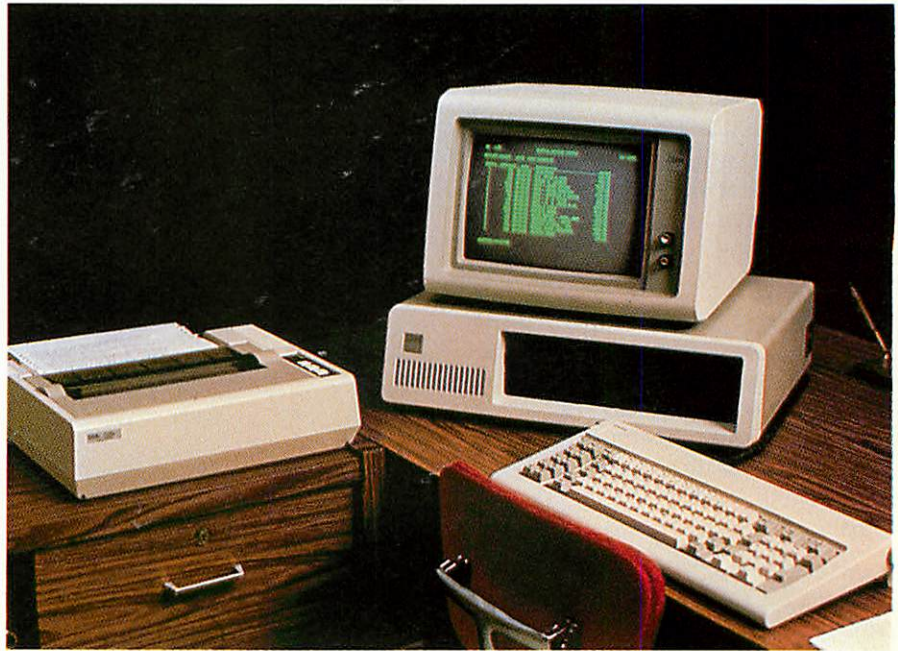
IBM Personal Computer console with disk drives, detached keyboard, printer, and monochrome monitor
