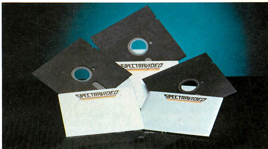
A floppy disk can store the equivalent of 25 to 40 typewritten pages of information on its magnetically coated surface.
