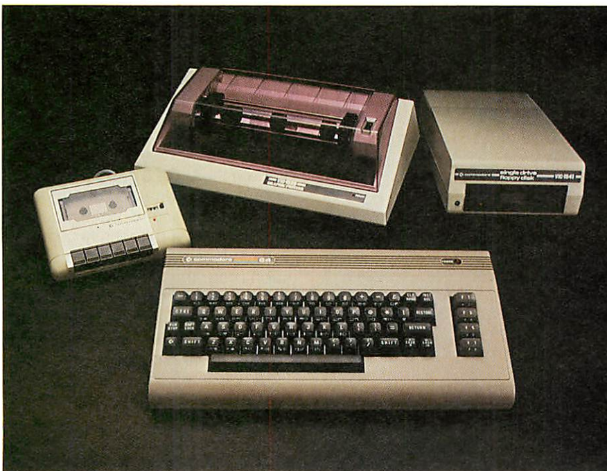
Commodore 64 computer, with the Commodore Datasette program recorder, graphic printer, and disk drive
