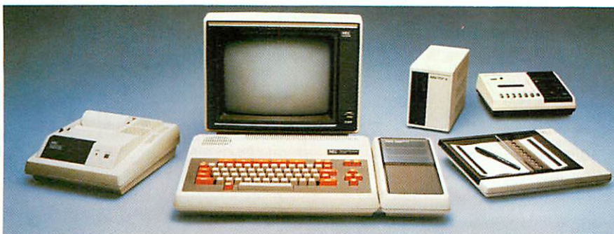
PC-6000 series computer, with NEC printer, color monitor, expansion module, disk drive, data recorder, and touch panel
